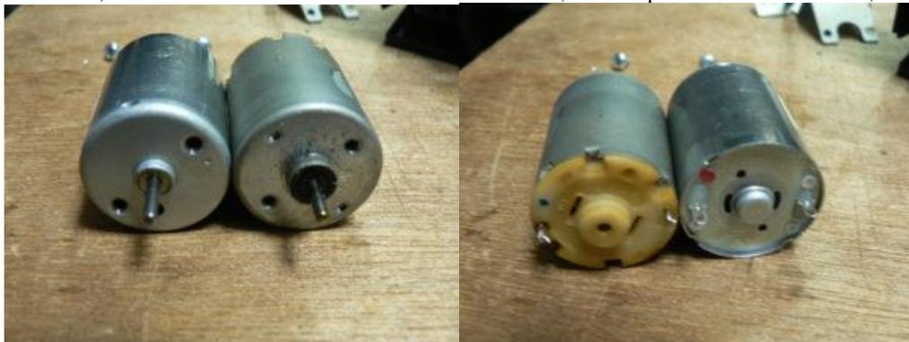
The sizes are almost the same, but the positions of the mounting holes and the size of the screws are slightly different.
