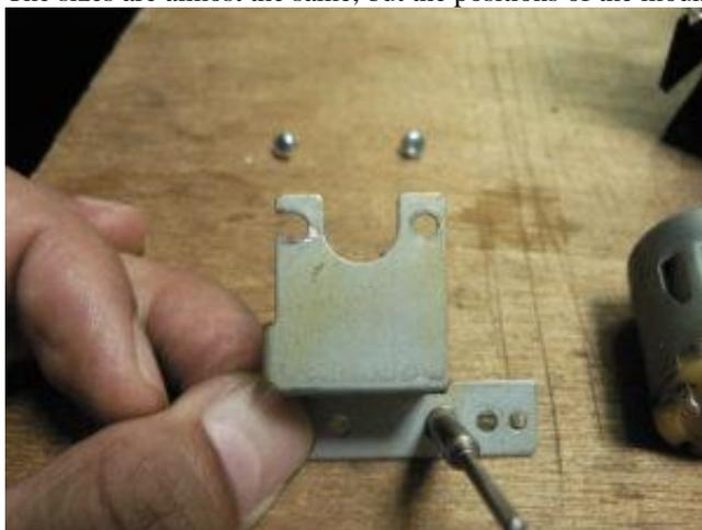
Therefore, some processing is required for the mounting part of the motor. Enlarge the hole (3 mm), change the mounting screw, and machine a long hole.
